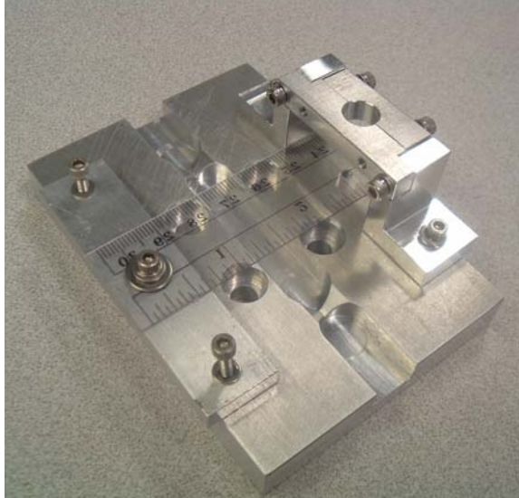
Figure A.21 The monocapillary bending platform used to dynamically bend single-bounce monocapillaries. An actuator (not shown) is put in the bracket on the right, which pushes on the plastic ruler. A monocapillary optic is placed in the V-groove, and a small sponge is placed between the optic and the plastic ruler. As the actuator pushes on the ruler, it in turn pushes on the sponge and then the optic to gently bend it. This is a modified version of the part shown in Figure A.15
