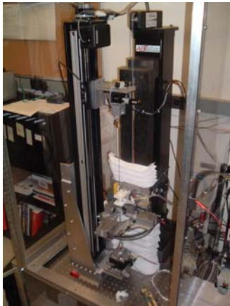
Figure 6.6 On the left is an image of the capillary puller. On the right is a diagram of the puller with the major components color-coded. The tension stage is in silver. The tension gauge, rotation motors, and the tension stage carriage are in green. The air/furnace stage is dark gray. The air stage carriage, the furnace, and the optical micrometers are in red.
