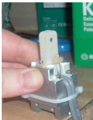
Figure A.17 An image of the small ion chambers available to use with the x-ray microbeam breadboard.
