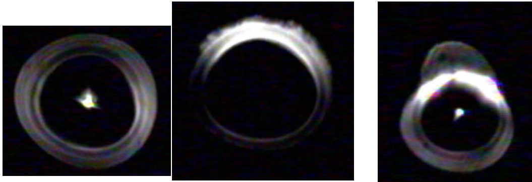
Figure 9.15 Three images showing the far-field patterns from moncapillary f1-mr9f20-02 taken at APS, beamline 18ID. The image on the left shows the entire far-field pattern (compare to f1b-mr9f20-01 in figure 4.4, an optic of the same design). The middle far-field pattern has the beam block in place. The ragged edge at the top of the far-field is due to the slightly oversize, non-ideal beam stop. The figure on the right shows the full far-field pattern after spending time in the undulator beam. Something has changed the optic's surface in that time.
