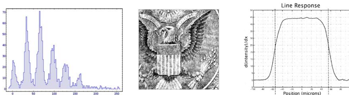
FIGURE 1. Left: Histogram of ADU/pix from single pixel illumination. Peaks from zero, one, two, ... five x-ray photons per acquisition are clearly seen. Middle: Radiograph of part of a U.S. dollar bill in \text{Cu K}_\alpha radiation. The green ink of the dollar provides the contrast. Right: The spatial response of the pixel shows that charge is only shared when the beam is \sim 20 \mu\text{m} from a pixel edge. In part, from [5].
