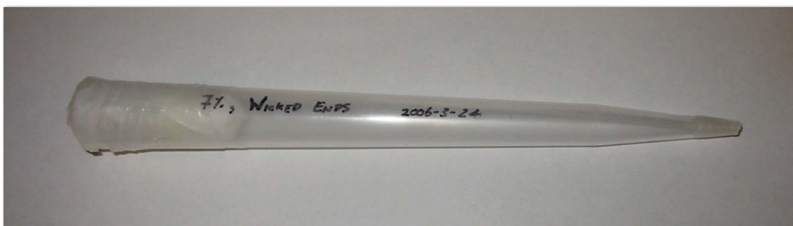
Figure 4.40: 10 mL pipette tip used for storing Citrine crystals grown in polycarbonate capillaries.
