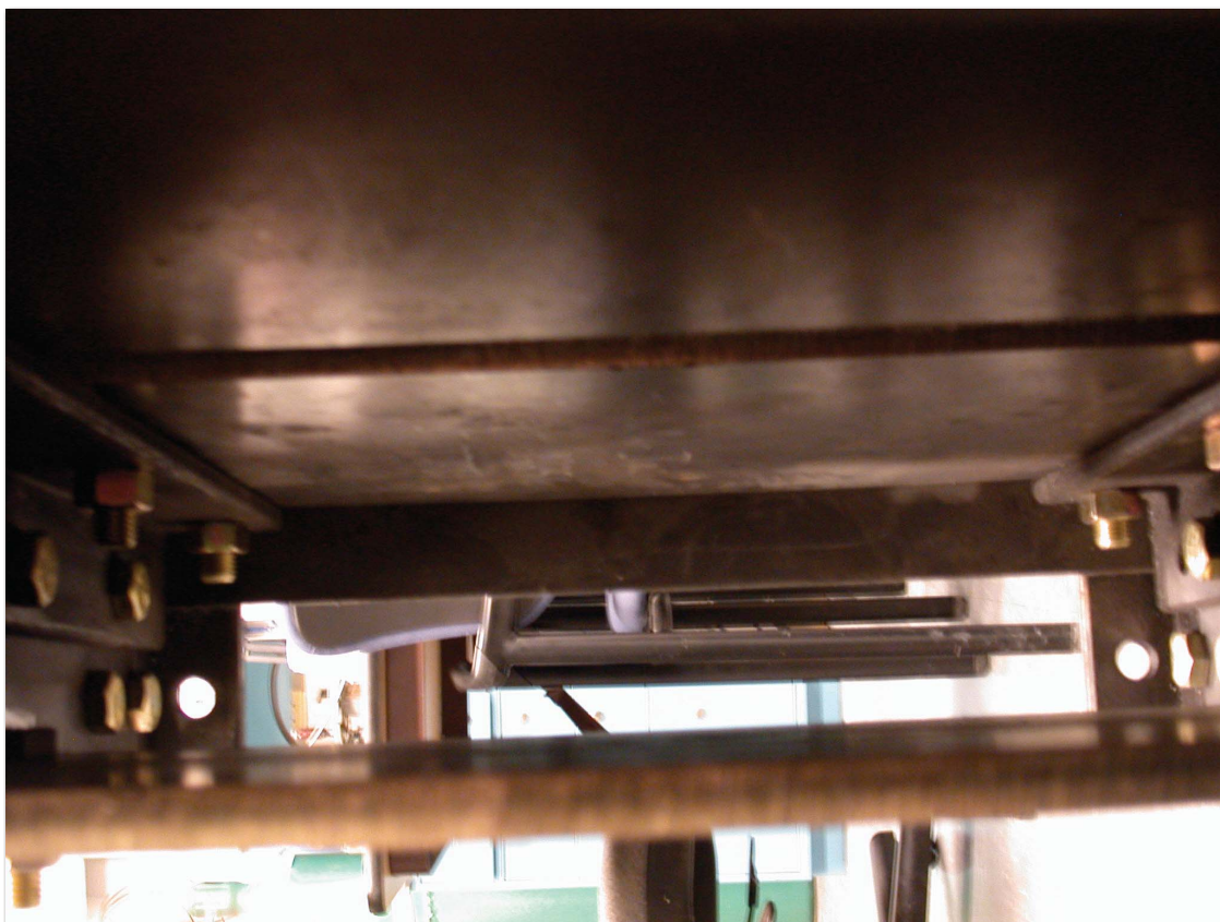
Figure 4.8: View of the gas exit port from the outside of the high-pressure cryocooling safety enclosure. Plate D (figure 4.7) is at the bottom of the photograph, and plates G and H are at the top of photograph.
