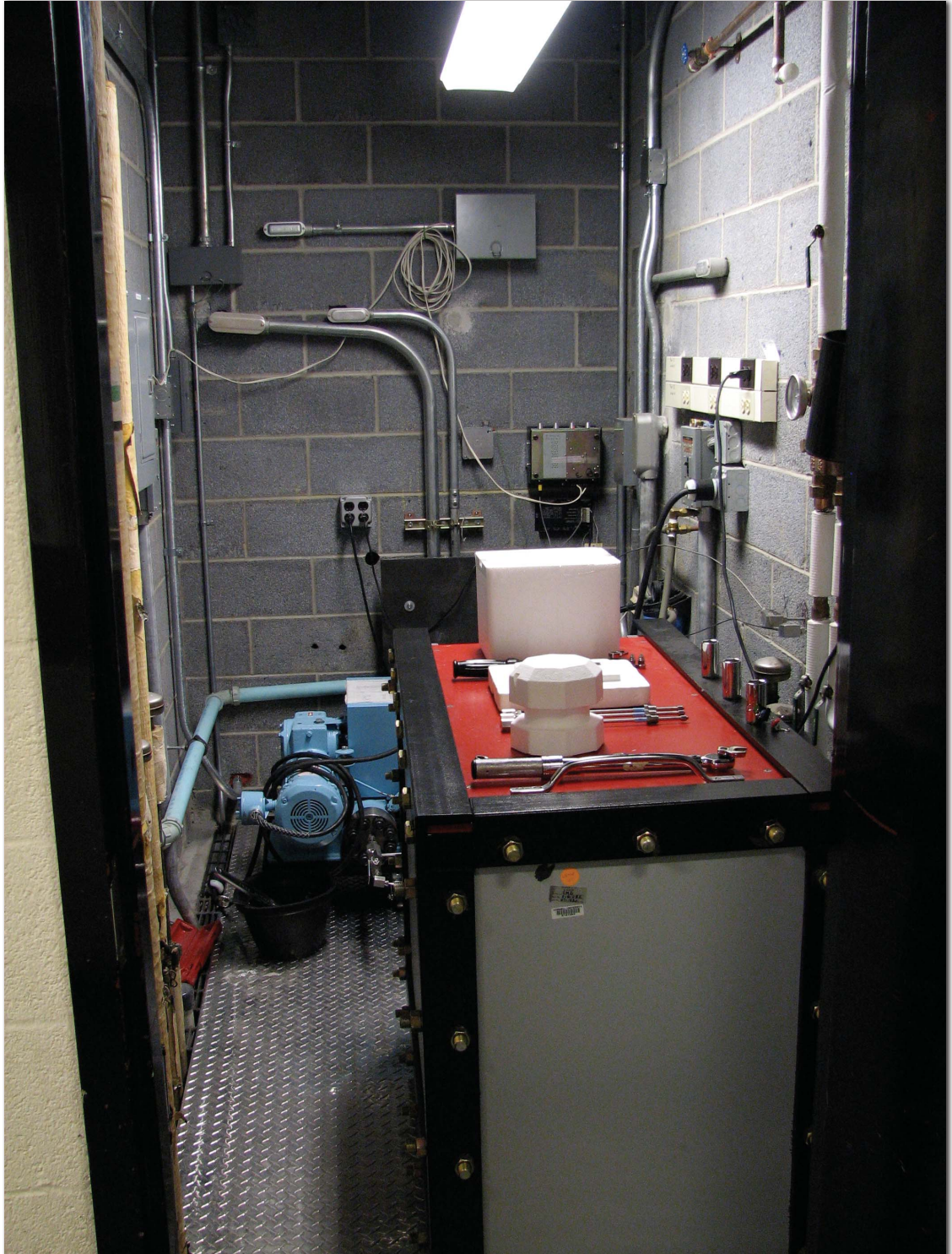
Figure 2.12: Photograph of high-pressure cryo-cooling apparatus after full assembly.
