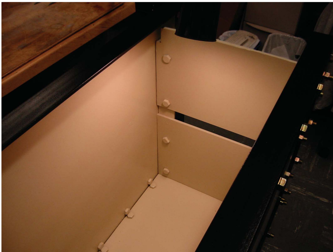
Figure 4.9: View of gas exit port (plates G and H in figure 4.7) from inside the high-pressure cryocooling safety enclosure.
