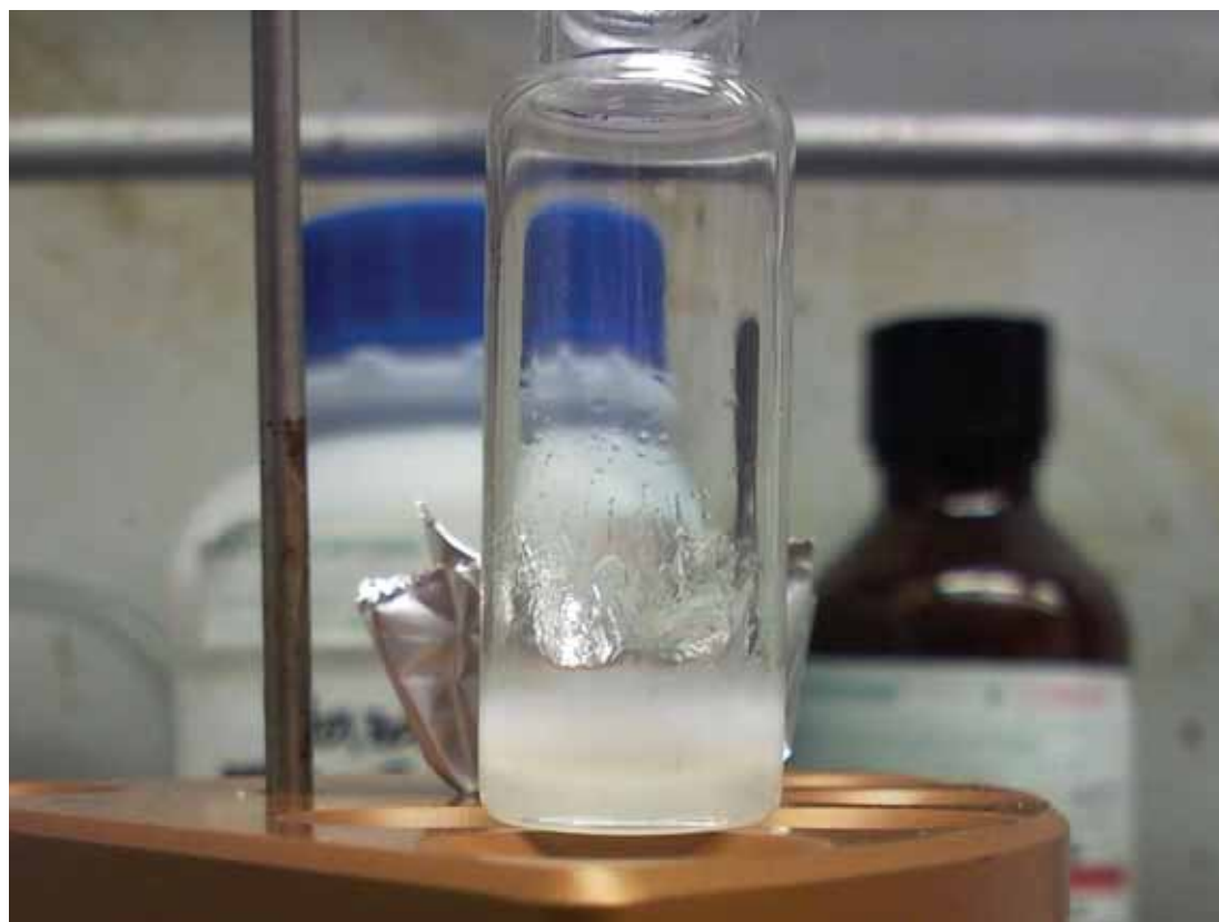
Figure 5.S1. Photograph of a PS- b -PEO/o-PEO mixture cast from xylene solution at 130 °C with the projected film thickness of 1 mm. Note the dual layer appearance in the vessel, where bottom layer is wet with solvent and top layer dense and dry.
