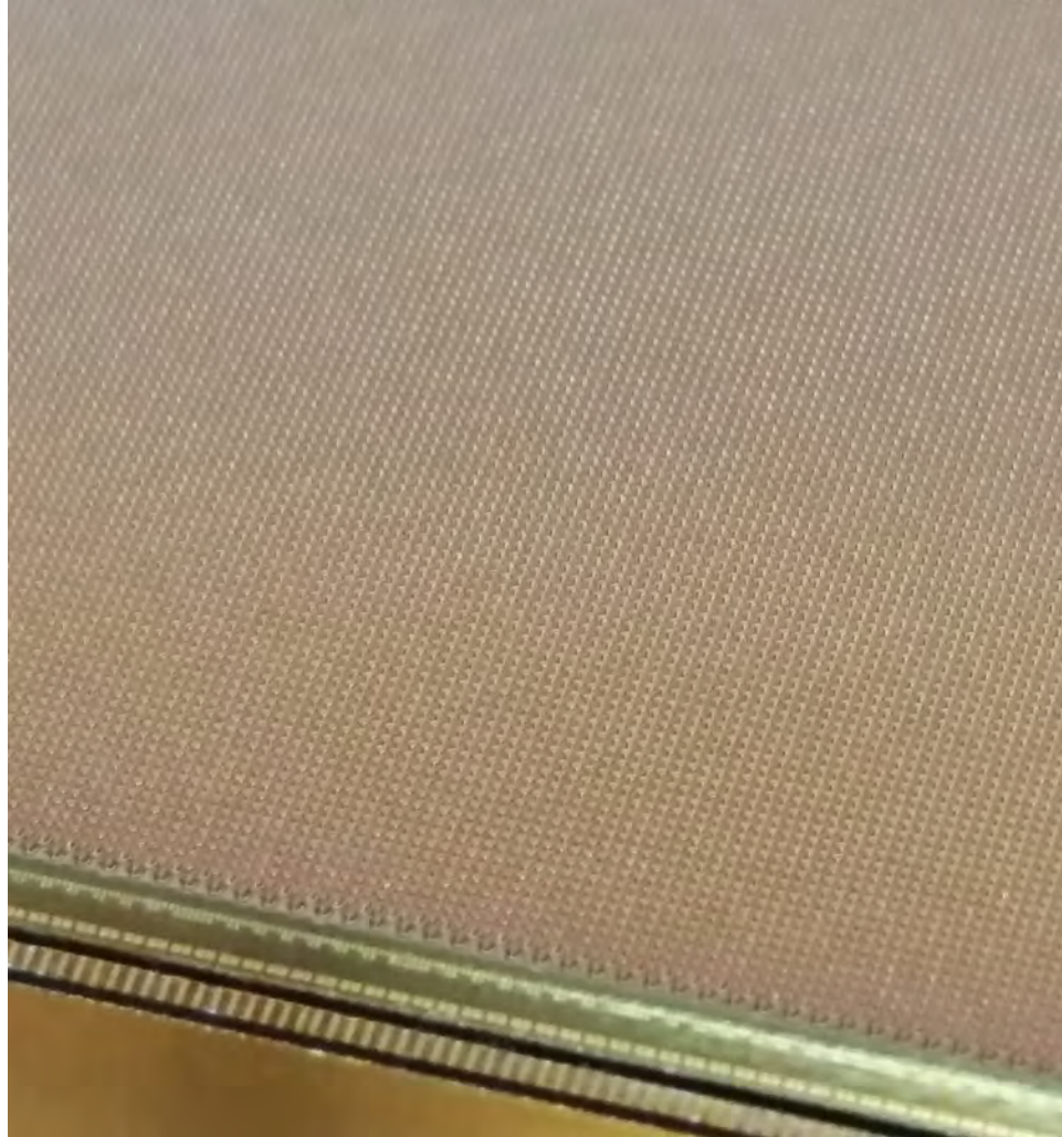
Figure 2.7: MM-PAD ASIC bump bonds. The ASIC contains a 128x128 array of solder bumps, one connected to each pixel, which can be bonded to a sensor with suitable backside metalization. Pixel pitch is 150 \mu m.
