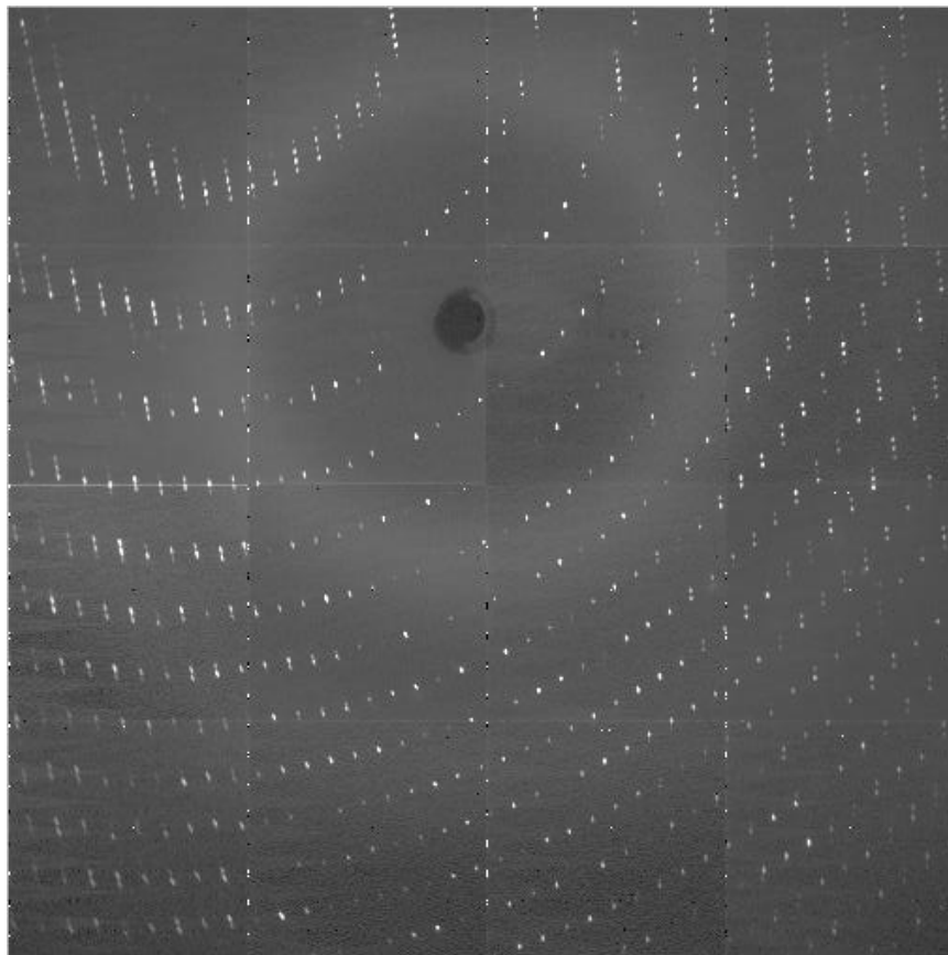
Figure 7.10: Mosaic image of the diffraction pattern from the Thaumatin protein crystal shown figure 7.9, when rotated through \Delta\phi = 1 deg. in 1 s. This image was made by combining sixteen separate images ( i.e. tiles) of the same crystal rotation, acquired with the same single PAD hybrid at sixteen different detector displacements. In each tile a separate background image was subtracted and the tiles global scaling was adjusted to offset beam intensity variation. The border evident at the edge of each tile is due to a one pixel overlap region between images. The data in this edge region is of poor quality due to the high edge leakage of the uncooled detector. This was the first protein diffraction pattern taken with the Mixed-Mode PAD. The image is shown to scale.
