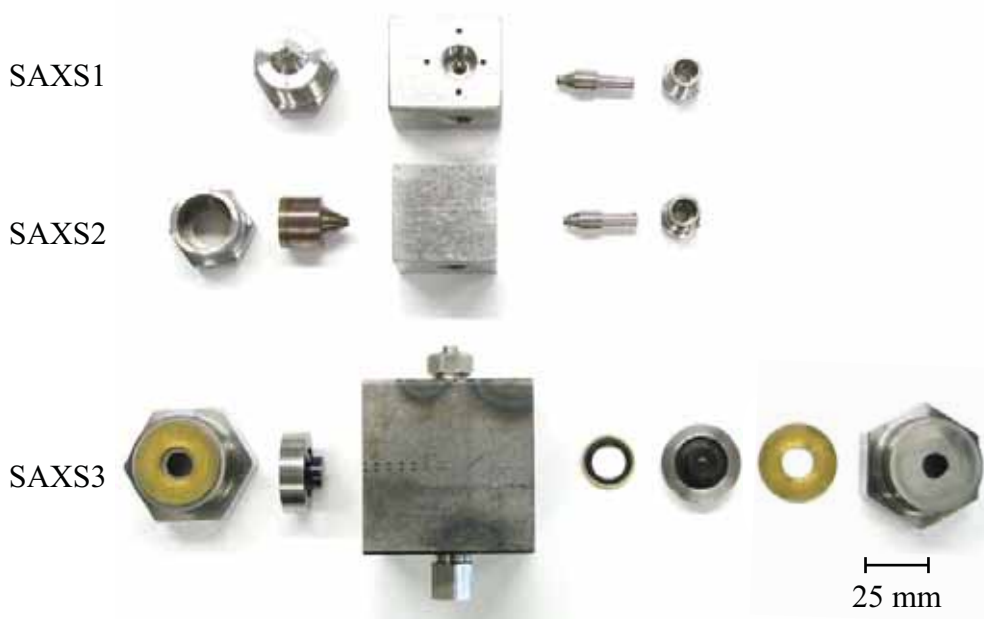
Figure 2.10: Three high-pressure SAXS cells designed for this thesis. The first-generation cells, SAXS1 and SAXS2, utilized cone seals for the window holders. The second-generation cell, SAXS3, features a corrosion-resistant Inconel body, window-retaining caps and robust seals for the window holders, enabling sample loading from the window port.
