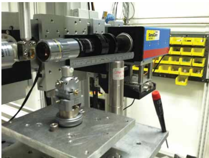
Figure 6.18: APS camera setup. From left: scintillator mount, microscope objective (silver), tube lens (black), camera body.
