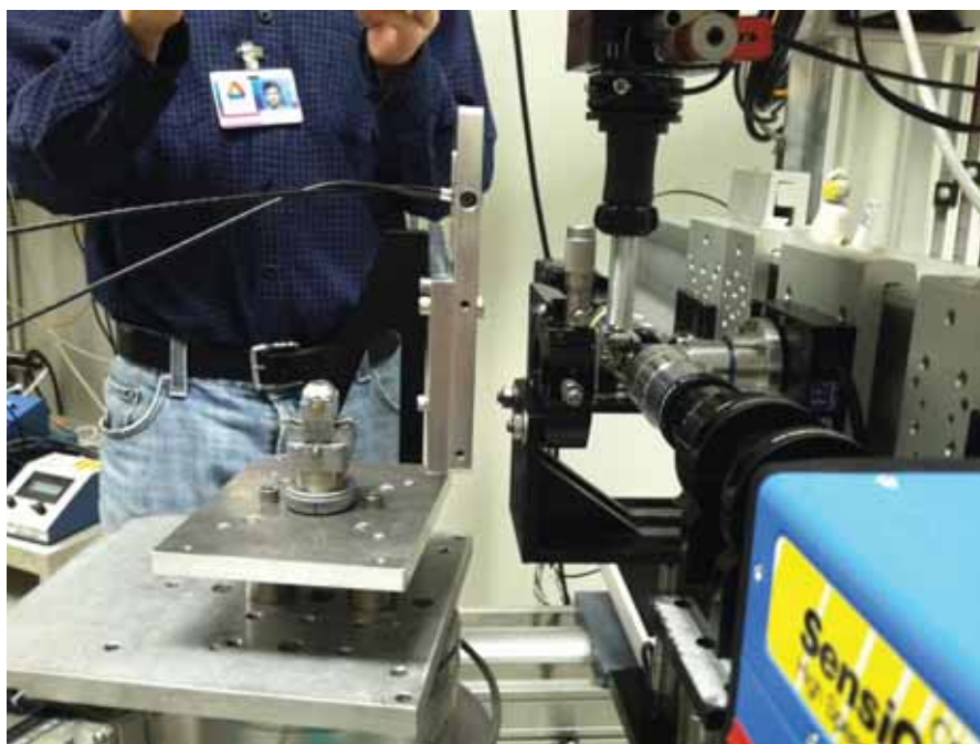
Figure 6.17: APS experimental setup. From left: goniometer mount for specimens, flexure stage, analyzer grating rotation stage, detector system. Upstream to the left of the image is the Uniblitz shutter.
