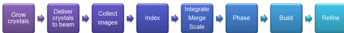
Figure 1.5: Simplified pipeline of traditional crystallography. First, protein crystals are grown from purified proteins in solution. They are delivered to the x-ray beam where they are imaged. The images are indexed to establish orientation, and datasets are integrated, scaled and merged together. The resulting intensity distribution is phased and a structure is built. Lastly, refinement cycles are performed to optimize the structure to the diffraction data. Each step is critical to be performed before moving onto the next in the traditional pipeline.
